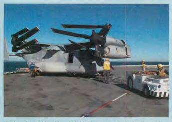
On board suitable ships, hybrid Osprey re-orients its fixed wing, folds its props/rotors for stowage.
